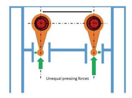
Large crank center distance (small main gears), Prevention of ram tilting cause of off center loading.
